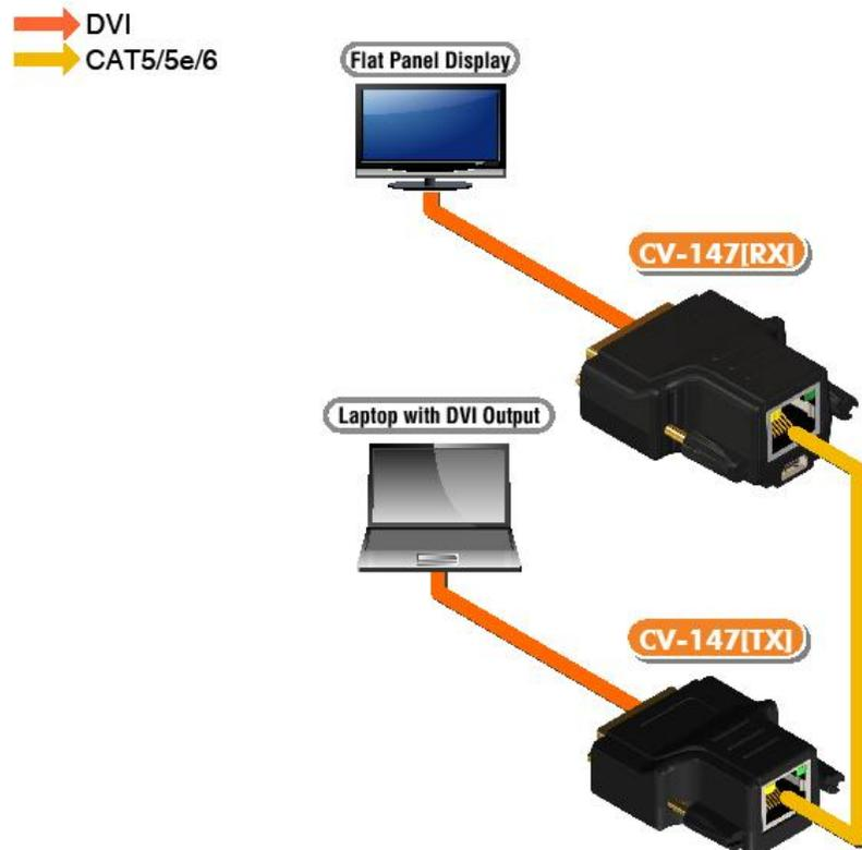
**i** 1. Most of the time, power will be unnecessary for CV-147, and it behaves exactly like its sister model CV-117! However, when encountering not enough current or voltage from DVI connection, CV-147 offers another path, USB, to compensate the deficiency of power supply!
